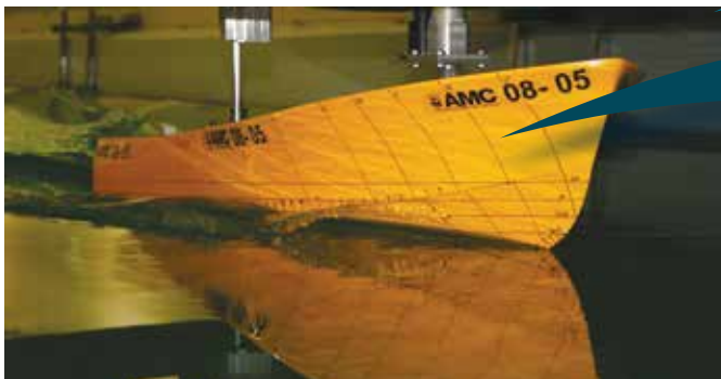
Hull resistance tests analyse speed/power ratios of full scale ships and craft
