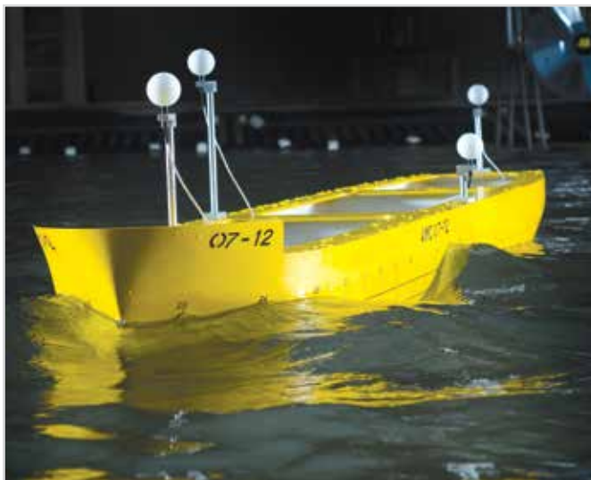
Measurement of vessel motions using a radio controlled model of a container ship in a seaway
