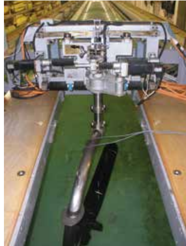
Horizontal planar motion mechanism predicts manoeuvring characteristics of vessels and underwater vehicles
