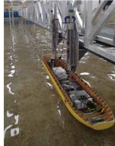
Model of a bulk carrier in the Model Test Basin to measure vessel squat and ship-bank interaction forces
